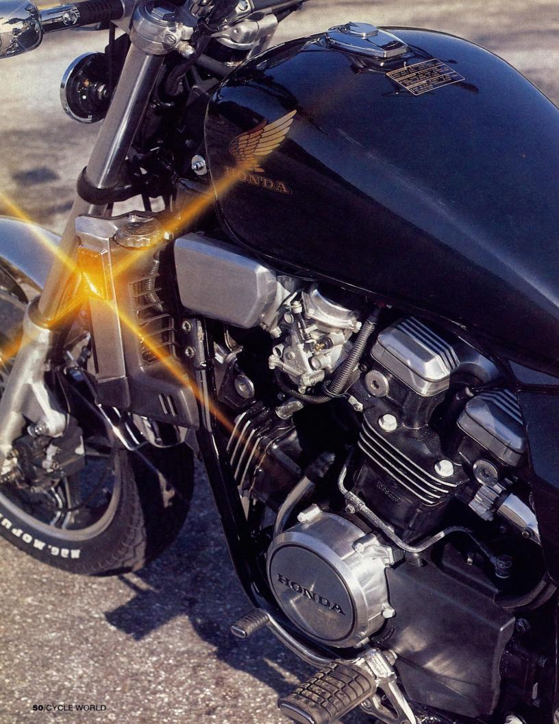
The Magna also reached 137 mph in a half mile; ran away from GPz and GS1100s in fifth-gear roll-ons from highway speeds; has a very tall sixth gear—Honda calls it an overdrive—that reduces rpm to 3500 at 60 mph and 5000 at 90 mph (redline is 10,000 rpm); and delivered 39 mpg on the Cycle World mileage test loop.
